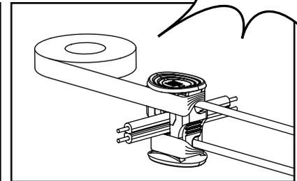
4.4 Once the clip-on connector is in place, wrap it with electrical tape for additional protection.
