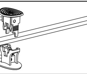
4.2 Align and fit the main low voltage cable vertically to the slot of wire connector as shown.
